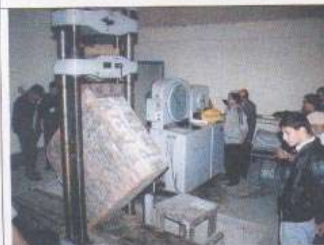
Testing of a 1.2 x 1.2 x 0.46 m non-reinforced-masonry-block prototype in Tribhuvan University Laboratory to obtain the diagonal tensional strength (shear strength) in masonry assemblies according to ASTM.
